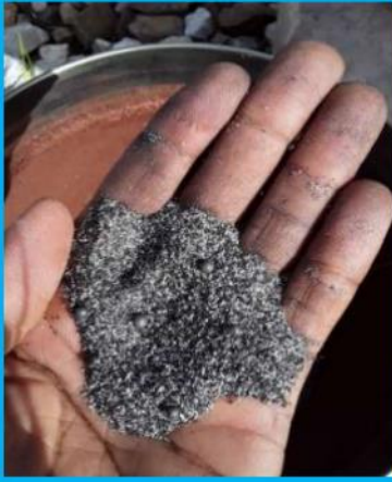
Thermite Welding. A Mixture of powdered Aluminum and Iron Oxide.
