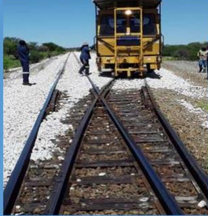
Other railway turnout/switch point. The railroad switch points help the train to be guided from one track to another. The switch points are one of the most interesting points on the railway system yet are complicated but beautiful at the same time.
